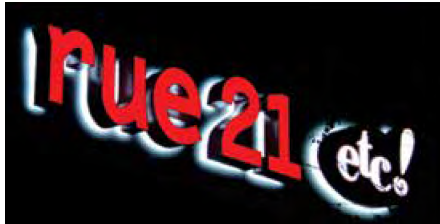
Face-Lit and Back-Lit "Halo" Combination LED Illumination
